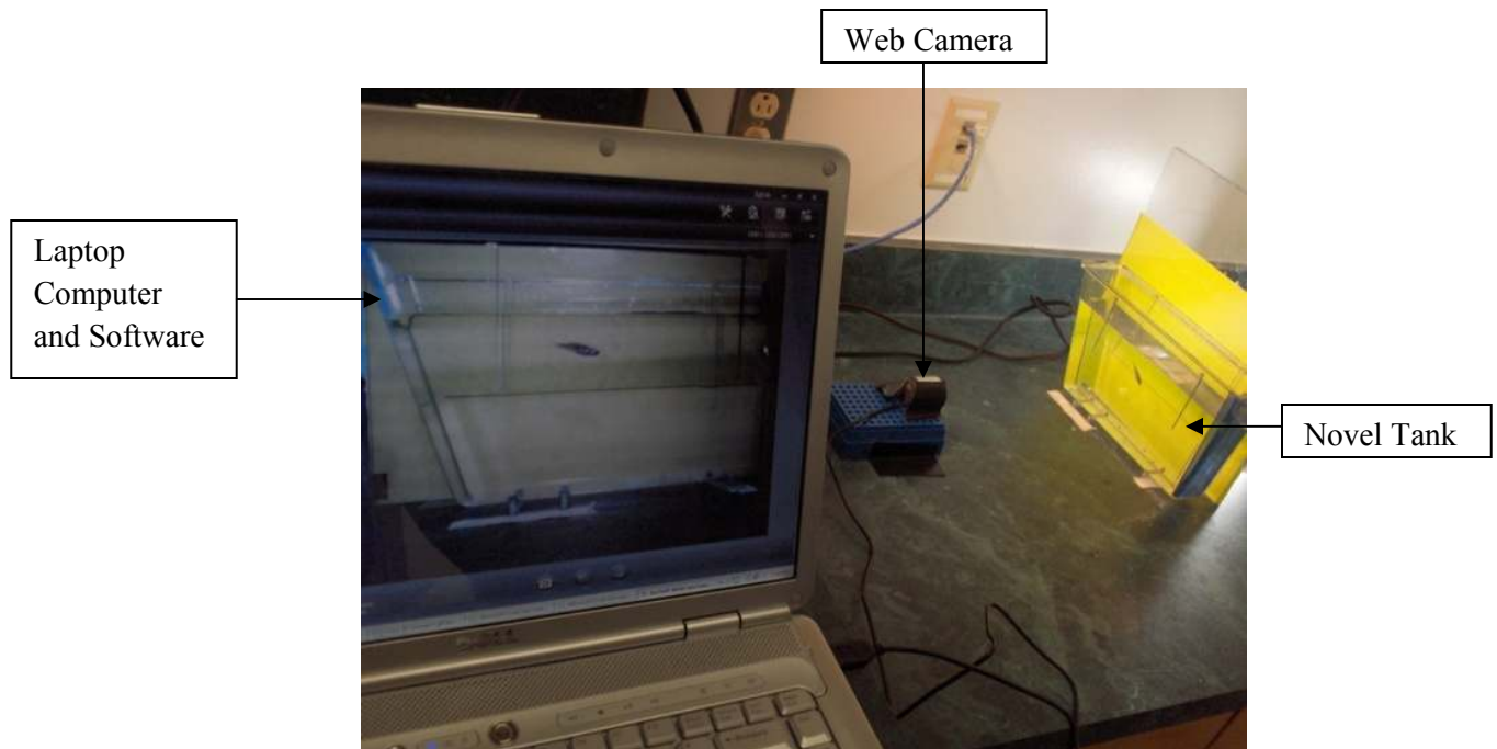
Figure 2: Zebrafish novel tank trial recording apparatus. Zebrafish are introduced to novel tank (right) for 6-min trial. Behavior was recorded on laptop (left) via webcam (center) for later analysis.
